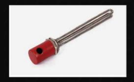
Industrial Water Immersion Heaters are made out of copper tube brazed to brass flange and are duly nickel plated. Each elements in provided with a brass check nut two fiber washers and a painted metallic cap with a' grommet for cable end.
